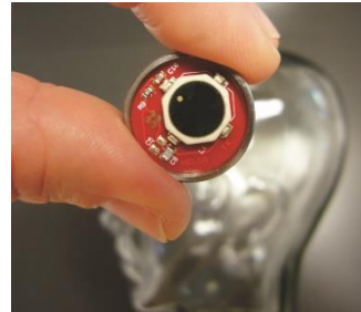
Micro Implant for long-term intracranial pressure monitoring.
